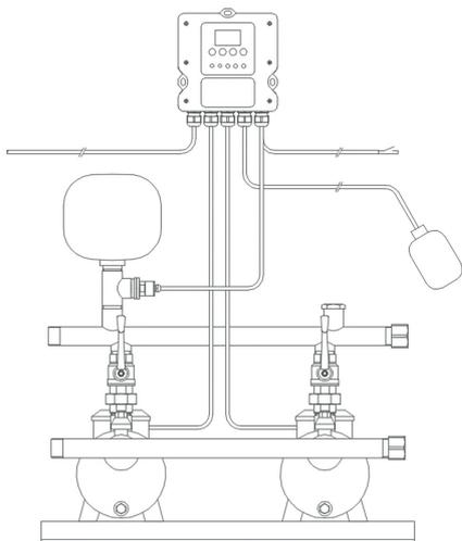
Use the three slots on the sides and top of the device to attach it to the wall, on the plate of a booster-set or hang it.
