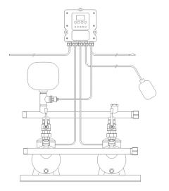
Use the three slots on the sides and top of the device to attach it to the wall, on the plate of a booster-set or hang it.
